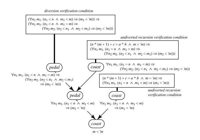
Leaves which duplicate the root produce *undiverted recursion verification conditions*.
