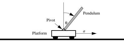
Let  $\theta \in U = [-5.0, 5.0]$  denote the current angle of the pendulum in degrees, with positive angles denoting clockwise from upright. Let  $a \in V = [-5.0, 5.0]$  denote the current acceleration of the platform in m/sec<sup>2</sup>, with positive accelerations to the right.
